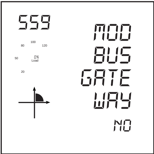
Figure 4-64 Modbus Gateway HMI Setting Page
