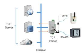
In TCP Client mode, the TCP Client initiates a TCP connection to the target IP address and port. If the connection fails, the TCP client will try to reconnect after the Reconnect Interval, until it succeeds. Afterwards, the RS-485enabled or LoRa devices communicate bi-directionally with the TCP server through the TCP client.
