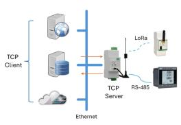
In TCP Server mode, the TCP Clients can initiate and establish the connection. The TCP Server shall listen to the specified Local IP Port and wait for the TCP client to connect. The data sent by the downstream RS-485-enabled or LoRa devices will be transparently transmitted to all successfully connected TCP clients by the TCP server.
