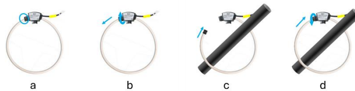
Figure 2-24 Rogowski Coil Installation Steps
