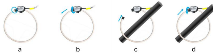
Figure 2-29 Rogowski Coil Installation Steps
