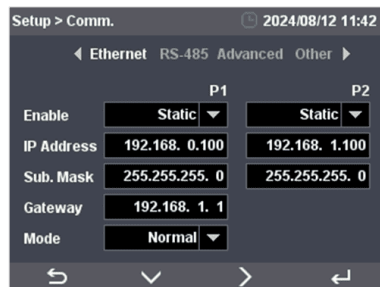
Ethernet Port Setup
