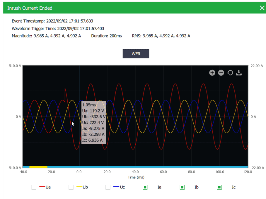
Figure 4-15 Inrush Current - displayed on Web Server
