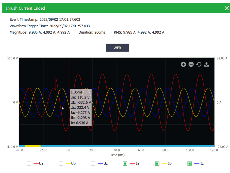
Figure 4-16 Inrush Current - displayed on Web Server
