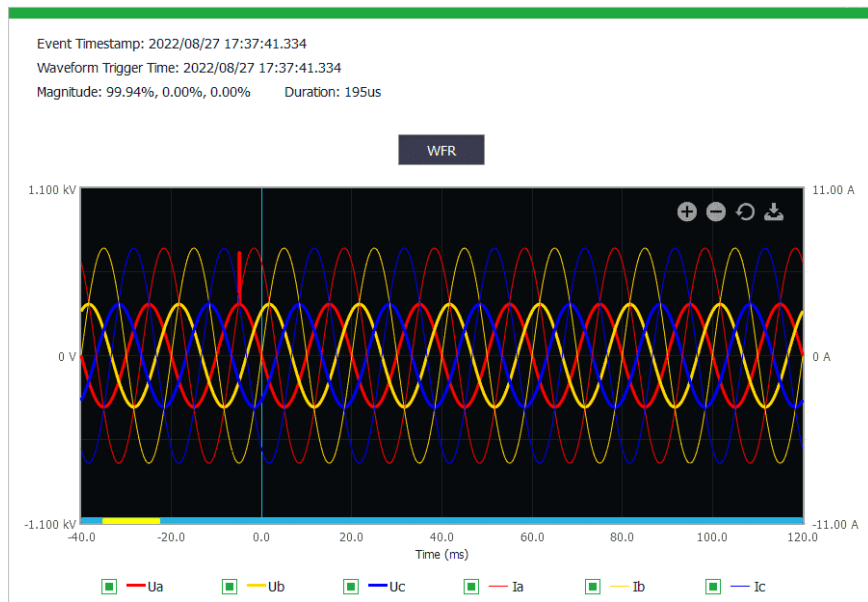
Figure 4-9 Transient Event @ 512 samples/cycle x 100 cycles
