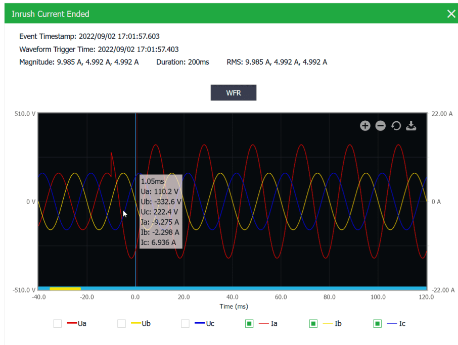
Figure 4-17 Inrush Current - displayed on Web Server
